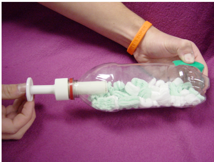
The styrofoam peanuts can compress to half their size and help students see the effect of high pressure in the bottle.
